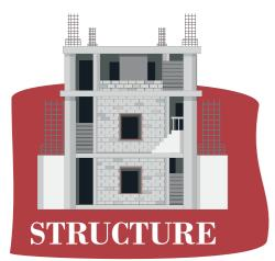
Column Foundation with framed structures with 9 and 41/2 brick walls The headroom of each floor will be 9'6" clear.
